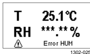
Figure 7 Measurement Screen with Error (HMD83D)
