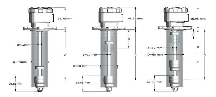
The dimensions A, B and C depend on the ordered version. For one signalling point: A min. 50mm, A max. 1000mm. For two signalling points: A min. 150mm, A max 1000mm; B min. 50mm, B max 900mm; (A – B) min. 100mm. For three signalling points: A min. 250mm, A max 1000mm; B min. 150mm, B max 900mm; C min. 50mm, C max 800mm; (A – B) min. 100mm, (B – C) min. 100mm.
